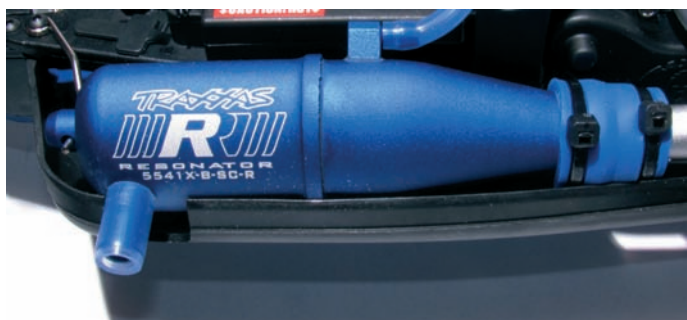
Above: The 'Resonator' tuned pipe offers a crisp note and an increase of power, note the Silicon sheath
