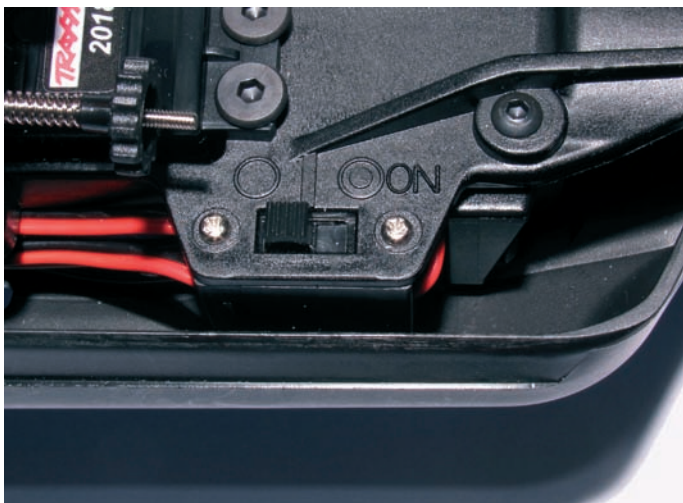
Above: The switch assembly is orientated to stay on in the event of an impact or as I call it 'rapid deceleration'
