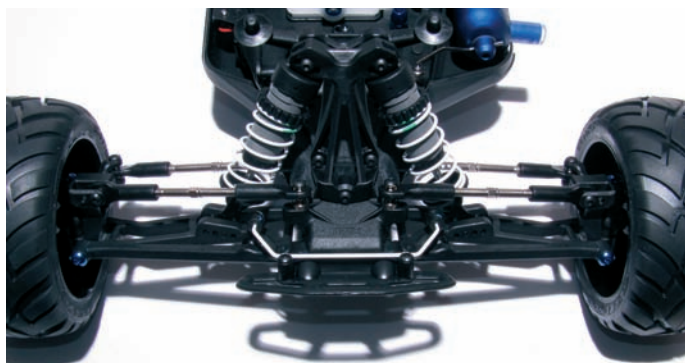
Above: Big bore shocks and sway bar as standard help keep the front end firmly planted in use
