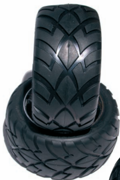
Left: Anaconda on road tyres have a large surface area and a tyre compound that offers bucket loads of grip
