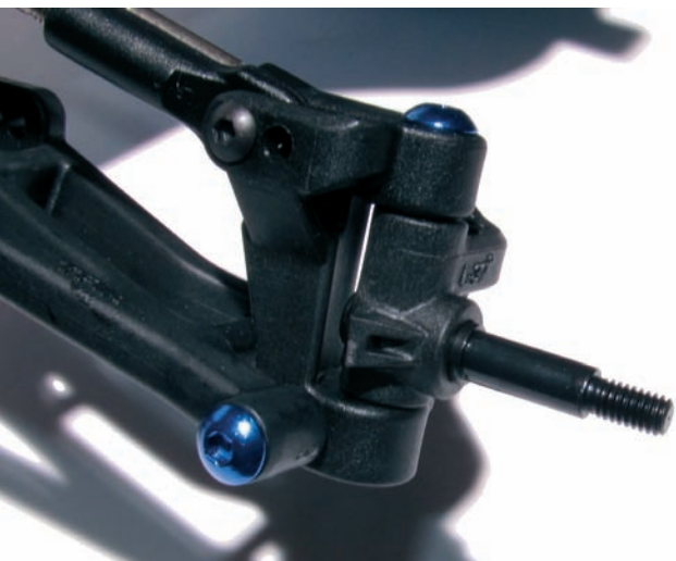
Below: C-Hub and steering knuckle design keeps things simple but effective!
