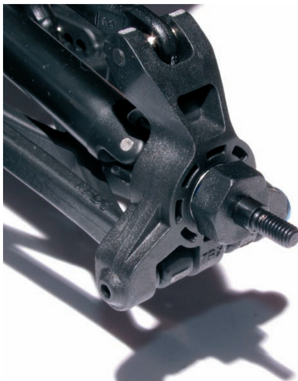
Above: Standard Hex's and tough plastic mouldings widen wheel choice and increase durability
