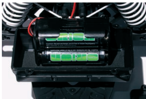
Above: We tried 4-cells initially, but a 5-cell hump pack offered better braking force, and faster steering response
