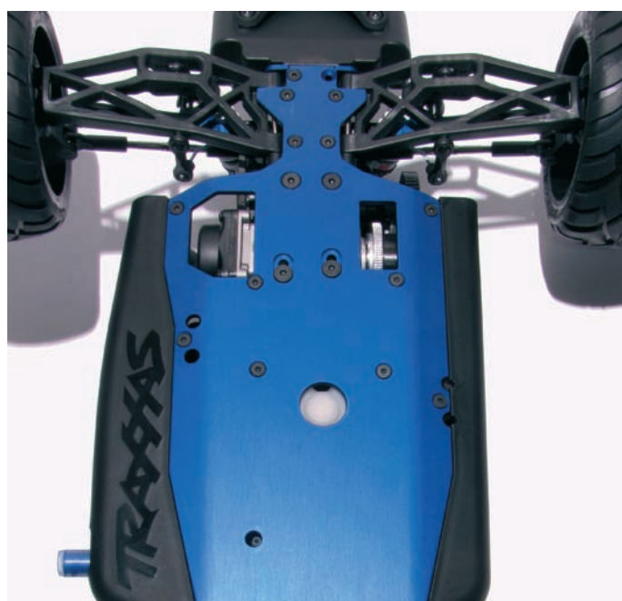
Above: A well designed chassis plate and hardened Hex hardware used throughout, again another Traxxas trademark
