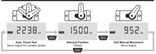
NOTE: If the servo you are testing is installed in a model, please be careful not to exceed travel limits as this may cause damage to your model and/or servo.
