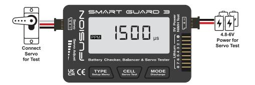
Connect the servo to be tested into the 'Servo Test PPM out' port. A long press on the 'Servo Test' button will enter the servo test function. Further short presses on the 'Servo Test' or 'Mode' buttons will scroll the different functions available:
