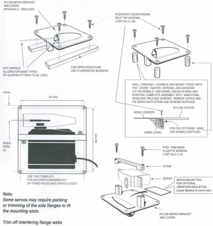
Trim off interfering flange webs where necessary, then sand or using a medium coarse file, reduce flange
