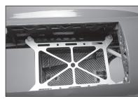
**102.** Use a wire tie to secure the fuel line to the clunk.
