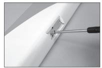
Place 2-3 drops of thin CA in each hole. Allow the CA to fully cure before proceeding.
