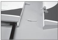
**34.** Install the control horn for the elevator using the techniques used for the aileron control horn.
