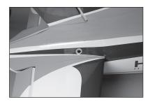
**133.** Mount the remote receiver above the fuel tank using hook and loop tape. Connect any extensions for the flaps, ailerons, retracts and brakes and route them back in the fuselage.
