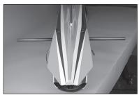
122. Mix 1/2 ounce (15ml) or 30-minute epoxy. Use an epoxy brush to apply epoxy in the tubes in the fuselage for the fin and to the surrounding wood.
