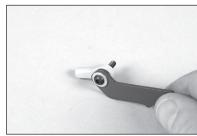
**20.** Remove the assembly and mix 1/2 ounce (15ml) of 30-minute epoxy. Apply epoxy in the control horn slots.
