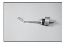
**98.** Check the bend in the tubing to make sure it does not touch the top of the tank.
