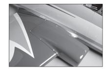
**146.** Use the screws and a 3mm hex wrench to attach the ventral fins to the bottom of the fuselage.
