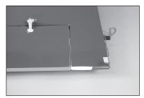
**25.** Check the operation of the flap to make sure there is clearance for the flap control horn. Use a rotary tool and sanding drum if necessary to lightly shape the opening in the wing for the control horn if necessary.
