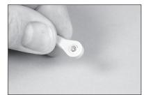
**18.** Fit the assembly into the slots in the aileron.
