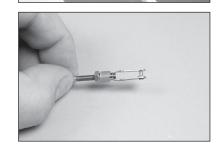
**60.** Remove any tape from the wing and flap. Assemble the flap linkage using two prepared ball ends and an 80mm threaded rod. Thread the ball ends equally on the threaded rod until the overall length is approximately  $4^{1}/_{4}$  inches (108mm).
