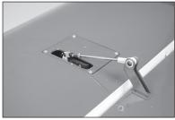
**53.** Apply 2–3 drops of thin CA in each hole to harden the surrounding wood. Allow the CA to fully cure before proceeding.
