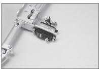
**81.** Prepare the retract mounting screws by sliding a 4mm lock washer, then a 4mm washer on the M4 x 20 socket head cap screws. Prepare all four mounting four screws.
