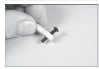
**19.** Place low-tack tape around the control horn base. This will help keep excess epoxy off the aileron.
