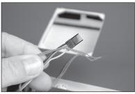
**44.** Apply 2–3 drops of thin CA in each hole to harden the surrounding wood. Allow the CA to fully cure before proceeding.
