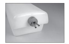
99. Use a soldering iron and solder to create an area on each of the tubes (both outside, and the unbent tube inside the tank) so the fuel tubing can be secured to the tubes.
