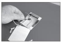
**45.** Mount the servo using the screws provided with the servo. Center the servo and attach the servo arm perpendicular to the servo centerline. Remove any arms that will interfere with the operation of the servo.
