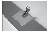
**15.** Slide an M3 washer on the M3 x 15 button head machine screw. Pass the screws into one of the control horns, then slide the ball end on the screw.
