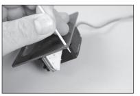
**51.** Place the aileron servo cover in position and drill through the mounting locations and into the wing using a pin vise and 1/16-inch (1.5mm) drill bit.
