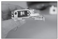
**88.** Fit the retract into the forward fuselage. Make sure all the leads are inside the fuselage and not between the retract frame and fuselage.
