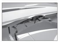
**132.** Secure the fuselage section using the five screws prepared earlier. Tighten the screws using a 3mm hex wrench.
