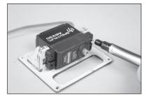
**46.** When connecting the clevis to the servo arm, use the hole that is 5/8 inch (16mm) from the center of the servo arm.
