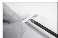
Apply a small amount of adhesive to each hinge where it will enter the flap and wing.
