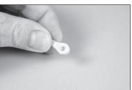
**54.** Secure the aileron servo cover using a #1 Phillips screwdriver and four M2 x 8 self-tapping screws.
