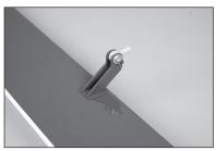
**14.** Slide an M3 x 15 button head machine screw into the ball. It may be necessary to use a small round file to remove any burrs from inside the aluminum ball. Prepare two ball ends.
