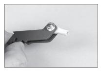
**12.** Test fit the aileron control horn. They should fit completely into the slot as shown. If they don't fit, use a file to open up the slot. Do not force the horn in with undue pressure.
