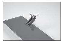
**39.** Use the same technique as the flap hinges to secure the rudder hinges. Make sure to remove any excess adhesive from the hinges using a paper towel and isopropyl alcohol. Use low-tack tape to hold the rudder in position until the adhesive has fully cured.
