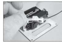
**43.** Thread a servo mounting screw into each hole, then remove the screws.
