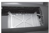
115. Space the exhaust tube equally between the sides of the fuselage. Secure the tube using four M3 x 12 self-tapping screws.
