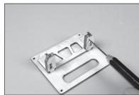
**47.** Secure a 12-inch (300mm) servo extension to the servo lead using a Servo Connector Clip (SPMA3054).
