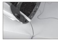
**121.** Use the string to pull the extension through the tube. Be careful not to break the string. Connect the lead from the rudder servo and extension using a commercially available retainer.
