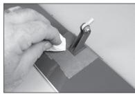
27. Inject adhesive into each of the hinge pockets of the wing.
