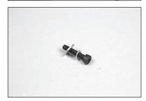
**86.** Assemble the steering linkage and attach it to the servo arm using an M3 x 15 button head screw, M3 washer and M3 lock nut. Use a 2mm hex wrench and 5.5mm nut driver.
