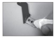
**16.** Slide the remaining control horn on the M3 x 15 button head machine screw. Secure the assembly using an M3 washer and an M3 locknut.
