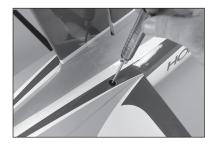
**128.** Insert the stabilizer screw grommet using a small amount of silicone adhesive.
