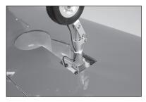
79. Route the brake lead and control lead from the retract into the wing.
