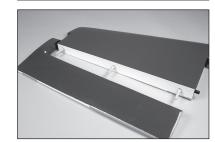
**38.** When installing the rudder hinges, note that the bottom hinge has been shortened to fit into the fin.
