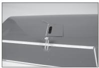
**41.** Place the aileron servo on the cover and use a felt-tipped pen to mark the locations for the mounting screws. The servo output will face forward.
