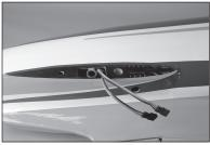
120. Wrap tape around the connection between the plug and string to make pulling the extension through the tube easier.
