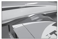
**138.** Use the two 1/4-20 x 2-inch nylon bolts to secure the wing to the fuselage.
