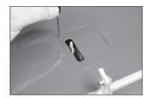
**56.** Remove the ball from the aileron control horn. Assemble the linkage so the overall length is 3<sup>3</sup>/<sub>4</sub> inches (95mm).
