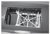
108. Slide the fuel tank into the fuselage. Use a small amount of silicone adhesive between the tray and tank to keep it from sliding on the tray during flight.
