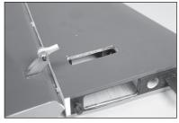
**74.** Mount the elevator servo in the stabilizer with the servo output facing forward.
