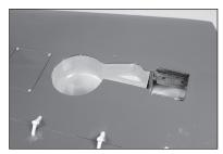
**83.** Check the operation of the retract using the retract module. A test button is located on the module, or the module can be connected to the receiver to check both the retract operation and the operation of the brake.
