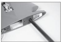
**131.** Slide the forward fuselage into position on the rear fuselage. They will fit tightly together.
