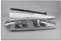
**80.** Retrieve the leads from the same location as the flap and aileron leads. Make sure to label the leads so they can be identified when assembling the model for flight.
