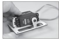
**50.** Use a toothpick or hobby knife with a #11 blade to puncture the aileron servo cover for the mounting screws.
