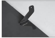
Slide the control horn base on the bottom of the control horn assembly.
