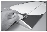
**35.** Use the same technique as the flap hinges to secure the elevator hinges. Make sure to remove any excess adhesive from the hinges using a paper towel and isopropyl alcohol. Use low-tack tape to hold the elevator in position until the adhesive has fully cured.
