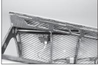
→ It may be necessary to use spacers under the retract frame to make sure there is no torsional stress when tightened into position. Torsional stress can cause intermittent operation of the retract unit.
