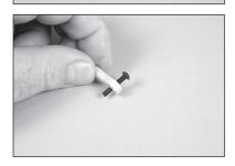
**55.** Slide a silicone retainer on the metal clevis. Thread the clevis on the 70mm threaded rod (on the end with the nut) until the end of the threaded rod is visible between the forks of the clevis.
