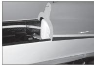
**114.** Align the end of the exhaust tube so it extends 1/4 to 1/2 inch (6mm to 13mm) beyond the fuselage former at the rear.
