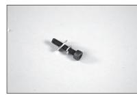
141. Use a pin vise and 1/16-inch (1.5mm) to drill to drill the locations in the intake into the wing. Remove teh intake and thread an M2 x 8 self-tapping screw into each hole. Remove the screws and place a drop of thin CA in each hole. Once the CA have fully cured, secure the intake to the wing using twelve M2 x 8 self-tapping screws.
