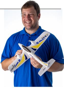
pilot better aware of approximately how much "power" remains while flying. Threechannel operation offers elevator (climb/descend), steering, and throttle control, while the twin electric motors deliver plenty of power plus differential thrust to turn.
