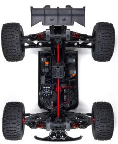
at 8.4V — nearly 50% more muscle than its predecessor. The new RTR package also includes a Spektrum FIRMA 160A V2 Smart ESC and Spektrum DX3 3-channel 2.4GHz DSMR radio system, with Spektrum AVC technology built-in to keep the huge power under control.
