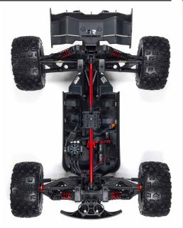
Spektrum FIRMA 160A V2 Smart ESC and Spektrum DX3 3-channel 2.4GHz DSMR radio system with Spektrum AVC technology built-in to keep the huge power under control.
