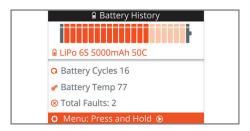
An integrated microchip allows each Smart battery to save vital information such as battery brand, chemistry, cell count, capacity, number of charging cycles, number of discharges, C rating, battery temperature, and internal resistance.
