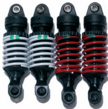
Above: The supplied white springs left and the harder red E-Revo ones I fitted right
