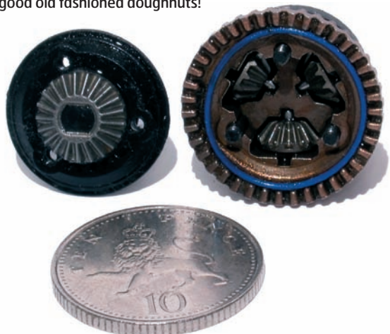
Above: Tiny gear diffs could be fine-tuned with grease or silicon oil
