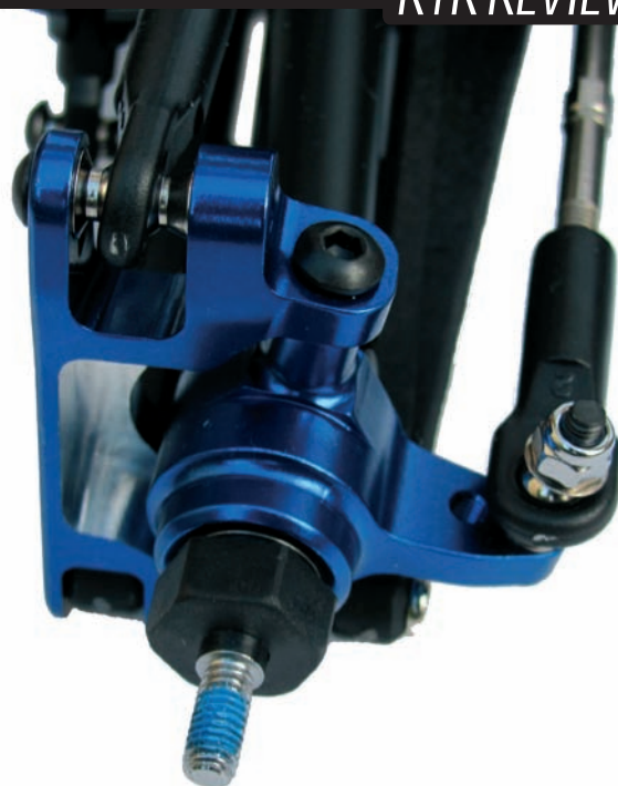
Above: Alloy C-Hubs and steering knuckles will take more abuse where it's really needed, without putting other components at risk
