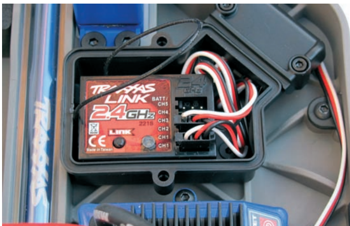
Above: The Traxxas Link 2.4 GHz receiver boasts twin steering channels and has 5-channel compatibility
