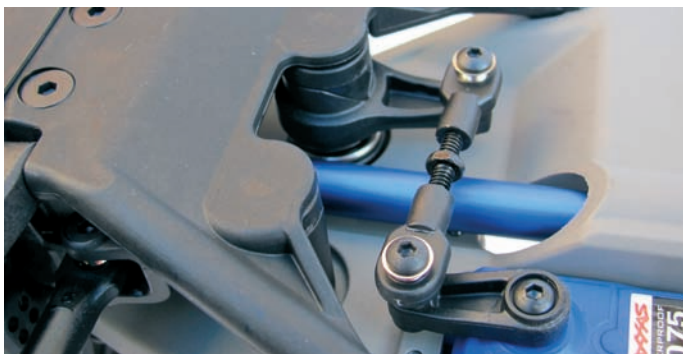
Above: Bellcrank steering offers direct and precise control, the steering servo protected by an adjustable servo saver
